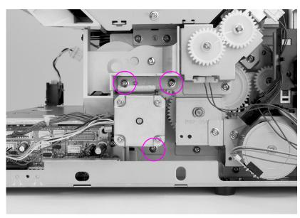
Figure 6-48 Fuser motor removal and replacement (2 of 2)
