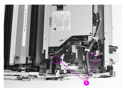
Figure 6-19 Top cover switch assembly removal and replacement
