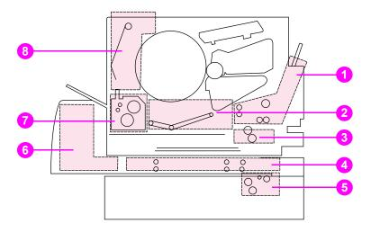
Figure 7-4 Jam locations (shown with the optional 500-sheet paper feeder and duplex unit installed)
