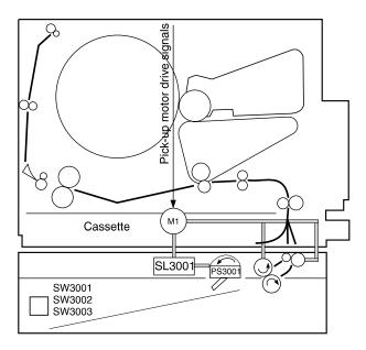
Figure 5-30 Pick-up and feed system
