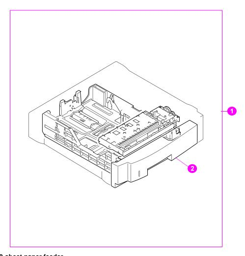
Figure 8-16 500-sheet paper feeder
