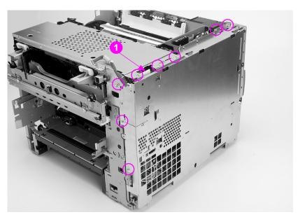
Figure 6-29 Formatter pan assembly removal and replacement (3 of 4)
