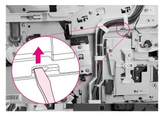
Figure 6-23 Drum drawer assembly removal and replacement (3 of 3)
