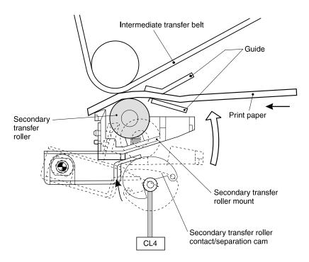
Figure 5-18 Secondary transfer roller unit
