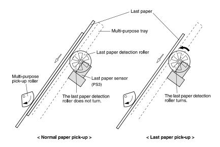
Figure 5-28 Laser paper detected
