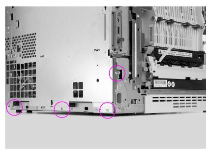
Figure 6-30 Formatter pan assembly removal and replacement (4 of 4)
