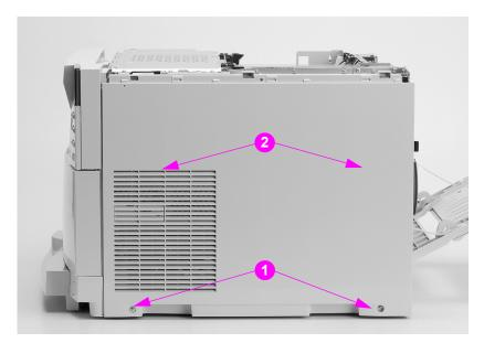
Figure 6-4 Right side cover removal and replacement
