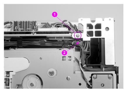
Figure 6-38 Large fan removal and replacement (2 of 2)
