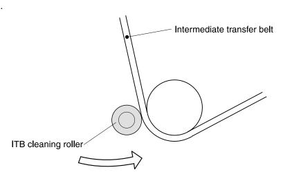
Figure 5-9 ITB residual toner cleaning
