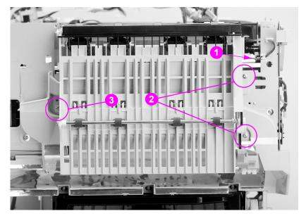
Figure 6-62 Rear paper path assembly removal and replacement
