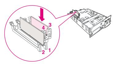
Figure 4-6 Do not remove the DIMM in slot #3.
