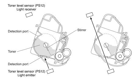
Figure 5-23 Toner level detection/toner cartridge detection
