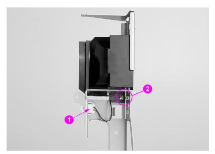
Figure 6-61 Left side fan removal and replacement (3 of 3)
