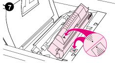
The cartridge slot for the black toner cartridge is visible. Lift up the flap that partially covers the cartridge slot. The correct toner color is shown on the flap.
