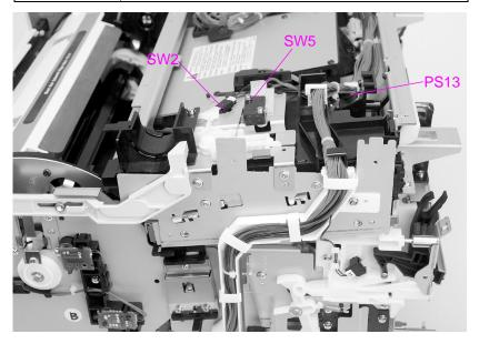
Figure 7-30 Miscellaneous switches and sensors
