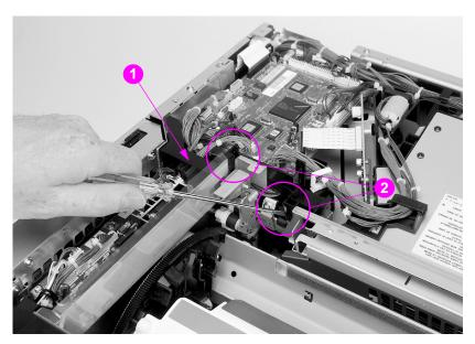
Figure 6-16 Developing PCB removal and replacement (1 of 2)
