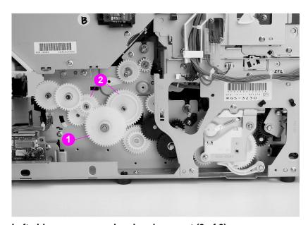
Figure 6-56 Left side gears removal and replacement (2 of 2)
