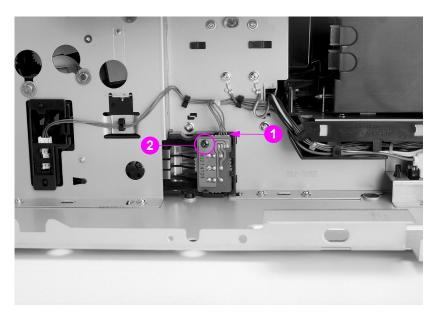
Figure 6-42 Paper size switch removal and replacement
