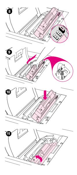
Make sure that the tab on the other end of the toner cartridge aligns with the notch on the cartridge slot.
