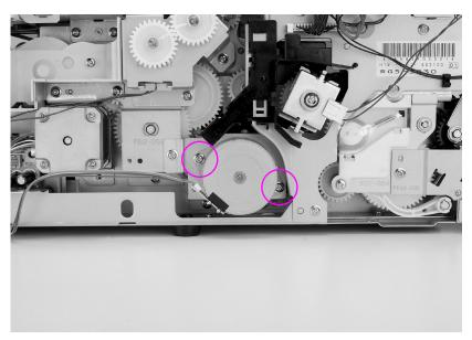
Figure 6-49 Paper path motor removal and replacement
