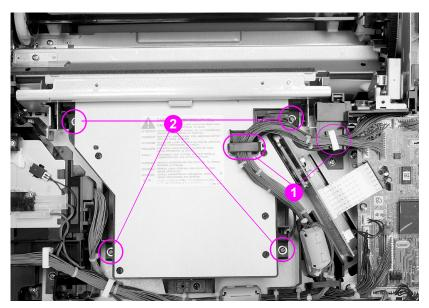
Laser/scanner assembly removal and replacement Figure 6-14
