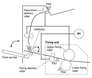
Figure 5-31 Fusing and delivery unit
