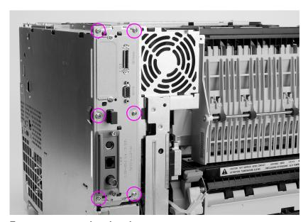
Figure 6-26 Formatter removal and replacement
