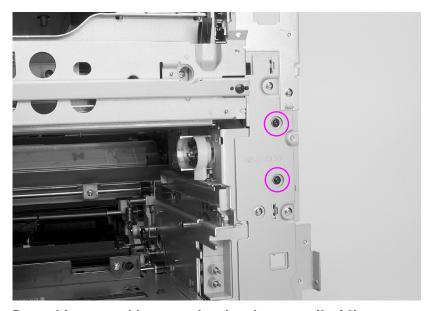
Figure 6-36 Drum drive assembly removal and replacement (3 of 3)
