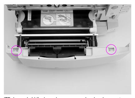
Figure 6-9 ITB drawer (middle drawer) cover removal and replacement
