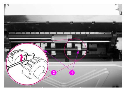
Figure 6-70 Paper pick rollers removal and replacement
