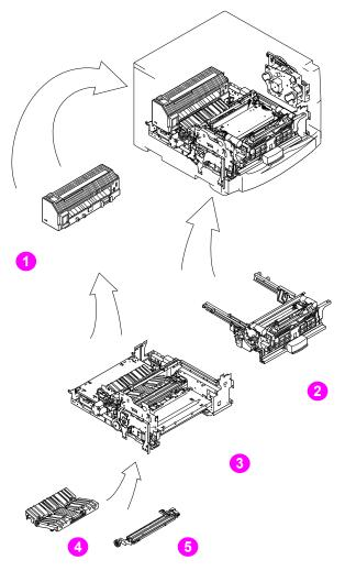
Figure 8-1 Assembly location diagram (1 of 2)
