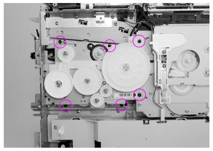
Drum drive assembly removal and replacement (2 of 3) Figure 6-35
