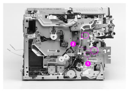
Figure 6-43 Switch plate assembly removal and replacement
