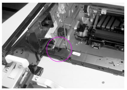
Figure 6-25 Densitometer removal and replacement (2 of 2)
