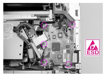
Figure 6-15 DC controller removal and replacement
