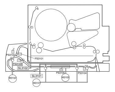
Figure 5-32 Reversing and duplex pick-up operation
