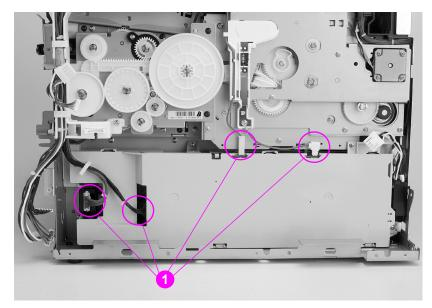
High-voltage power supply removal and replacement (older version HP Color LaserJet 4500 Figure 6-33 printers)
