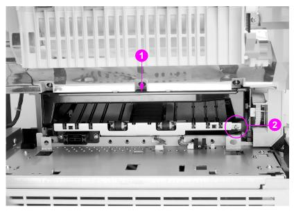
Figure 6-69 Paper transport assembly removal and replacement
