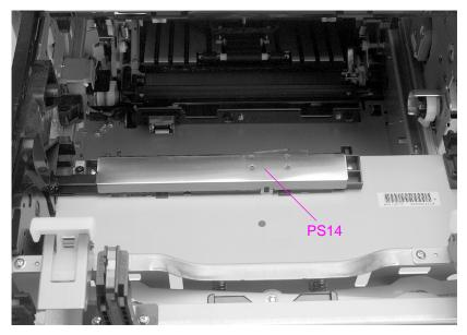
Figure 7-31 PS14 sensor location
