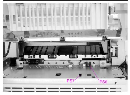
Figure 7-28 PS6 and PS7 sensor location
