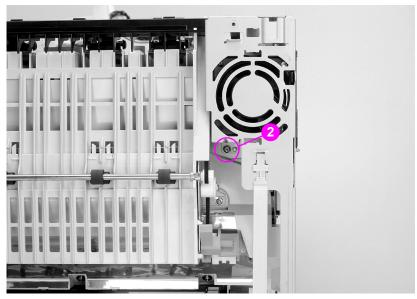
Figure 6-60 Left side fan removal and replacement (2 of 3)
