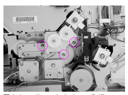
Figure 6-53 ITB clutch assembly removal and replacement (2 of 2)
