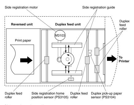
Figure 5-34 Side registration adjustment
