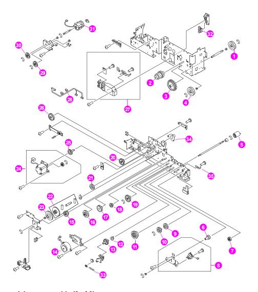
Figure 8-11 Paper pick-up assembly (2 of 3)
