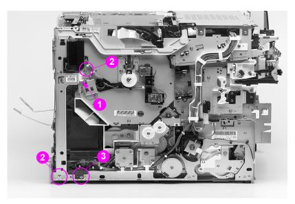
Figure 6-44 Paper feed PCB removal and replacement (1 of 3)
