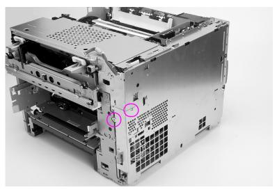
Figure 6-27 Formatter pan assembly removal and replacement (1 of 4)
