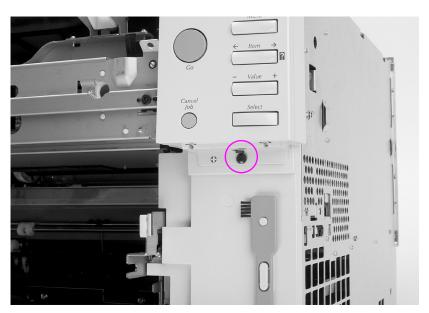
Figure 6-11 Control panel removal and replacement
