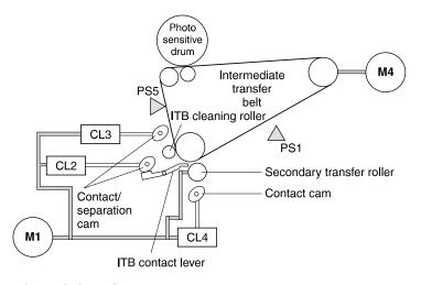
Figure 5-15 **Transfer unit function**
