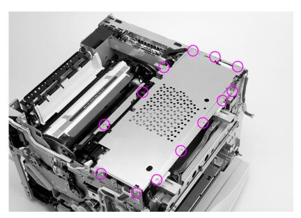
Figure 6-13 RFI shield removal and replacement
