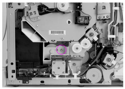
Figure 6-52 ITB clutch assembly removal and replacement (1 of 2)
