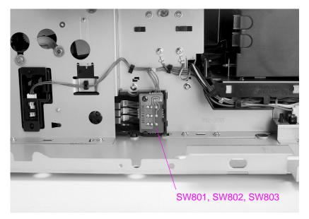
Figure 7-29 Miscellaneous switches
