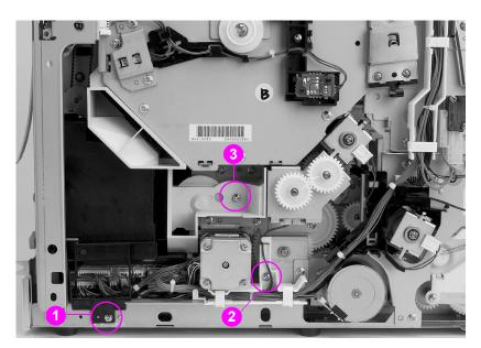
Fuser motor removal and replacement (1 of 2) Figure 6-47
