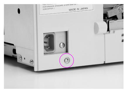
Figure 6-6 Right rear cover removal and replacement
