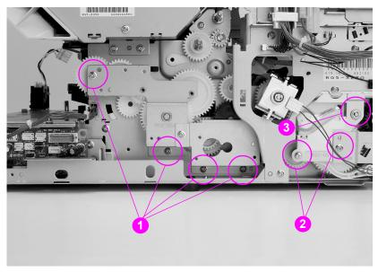
Figure 6-55 Left side gears removal and replacement (1 of 2)
