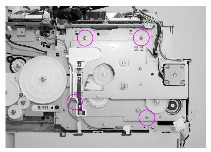
Figure 6-41 Carousel drive assembly removal and replacement (2 of 2)
