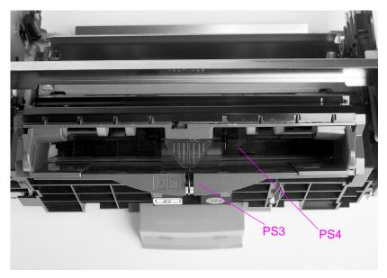
Figure 7-27 Miscellaneous sensors (with tray 1 front cover removed)
