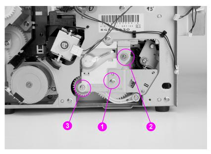
Figure 6-50 Paper pick solenoid removal and replacement
