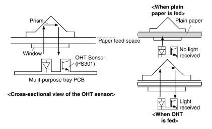
Figure 5-29 Overhead transparency sensor
