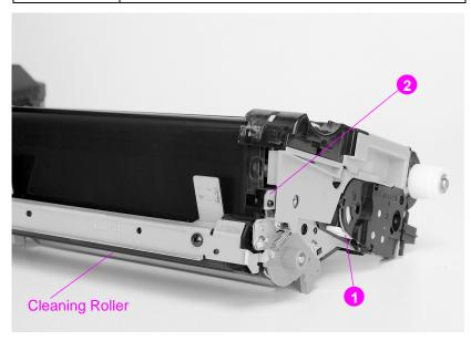
Figure 7-26 Intermediate transfer belt sensors
