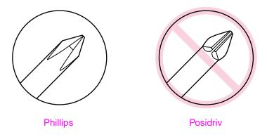
Figure 6-1 Phillips and Posidriv screwdriver comparison
