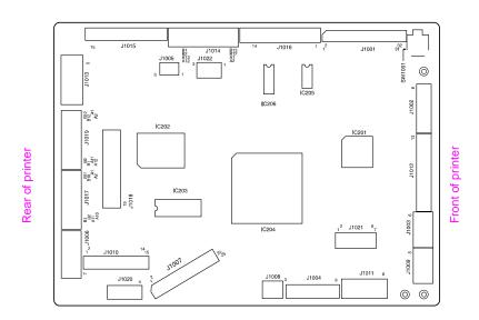
Figure 7-38 DC controller PCB connectors
