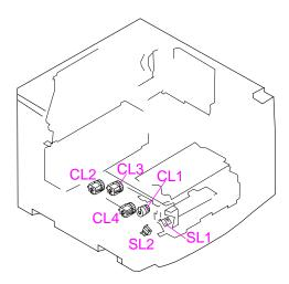
Printer solenoids and clutches Figure 7-23
