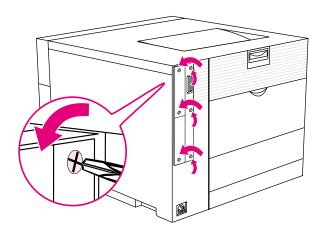
Figure 4-4 Removing the formatter board
