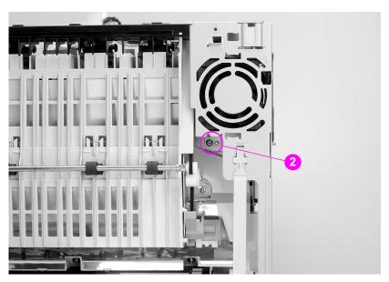
Paper feed PCB removal and replacement (2 of 3) Figure 6-45
