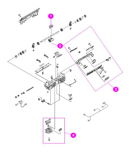
Figure 8-14 MP tray paper pick-up assembly
