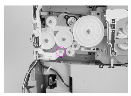
Figure 6-34 Drum drive assembly removal and replacement (1 of 3)
