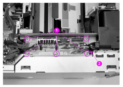
Figure 6-17 Developing PCB removal and replacement (2 of 2)
