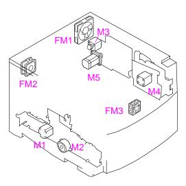
Figure 7-24 Printer motors and fans
