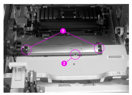
Figure 6-24 Densitometer removal and replacement (1 of 2)
