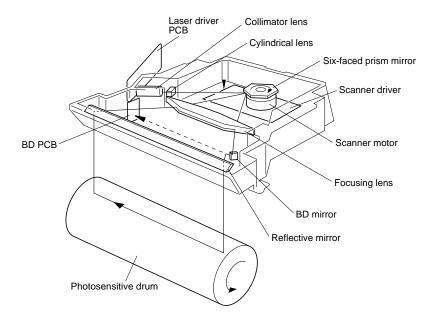
Figure 5-24 Laser/scanner operation
