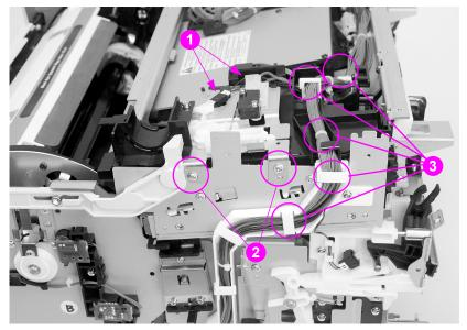
Figure 6-18 Top cover switch assembly removal and replacement
