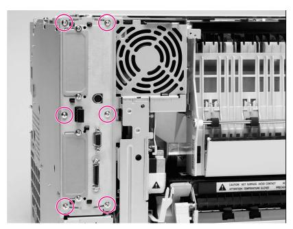
Figure 6-63 Cartridge carousel replacement - formatter pan assembly (1 of 6)
