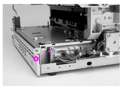
Figure 6-46 Paper feed PCB removal and replacement (3 of 3)
