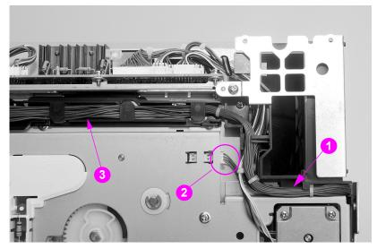
Figure 6-40 Carousel drive assembly removal and replacement (1 of 2)
