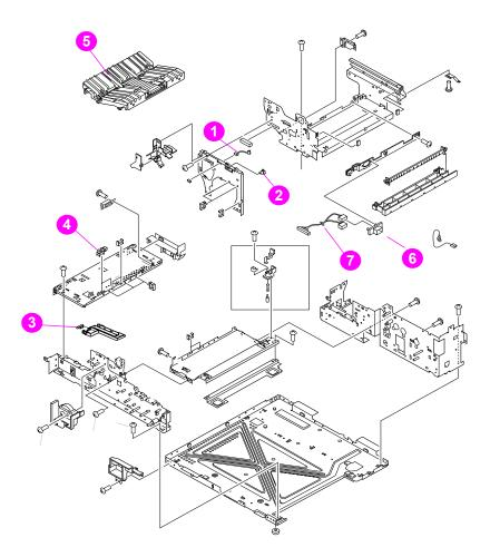
Figure 8-10 Paper pick-up assembly (1 of 3)
