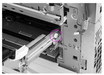
Figure 6-10 ITB drawer (middle drawer) removal and replacement
