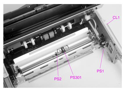
Figure 7-25 Miscellaneous sensors and clutches
