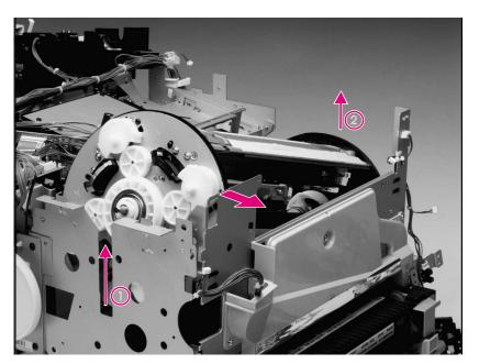
Cartridge carousel replacement - lift out the cartridge carousel (6 of 6) Figure 6-68
