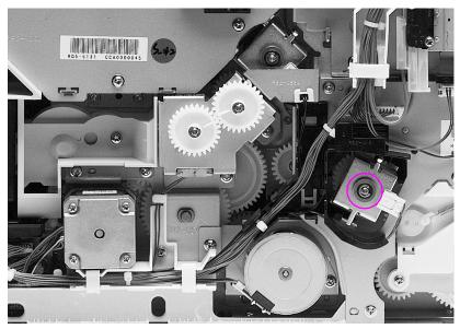
Figure 6-54 Transfer roller cam clutch removal and replacement
