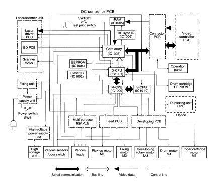
Figure 5-36 DC controller PCB
