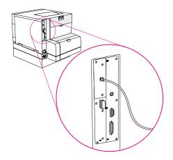
HP Color LaserJet 4550 RJ-45 (10Base-T or 10/100Base-TX) connection
