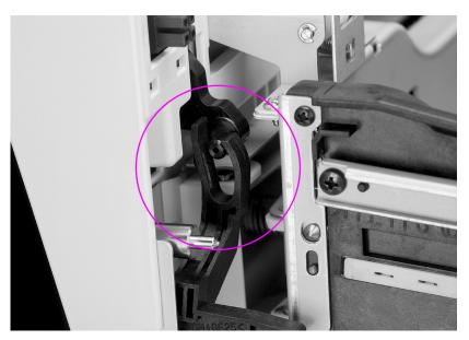
Figure 6-8 Drum drawer (top drawer) cover tabs and levers
