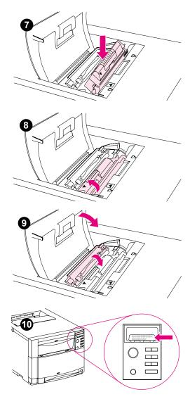
Slide the toner cartridge down into the slot until the cartridge 7 stops.
