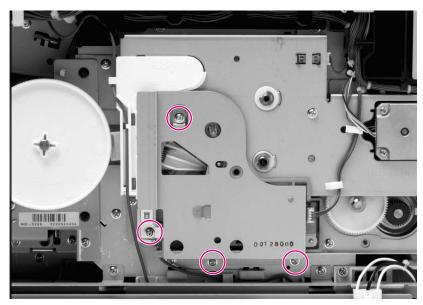
Figure 6-39 Toner level sensor assembly removal and replacement
