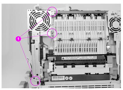
Figure 6-37 Large fan removal and replacement (1 of 2)
