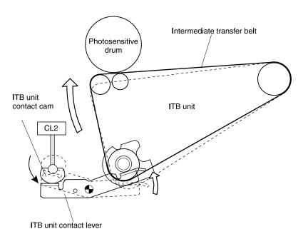
Figure 5-19 ITB unit contact/separation unit
