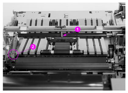
Figure 6-71 Star wheel assembly removal and replacement
