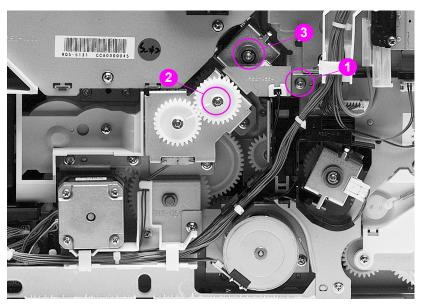
Figure 6-51 ITB cleaning roller clutch removal and replacement
