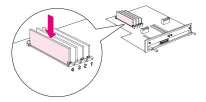
Figure 4-5 Do not remove the DIMM in slot #4.
