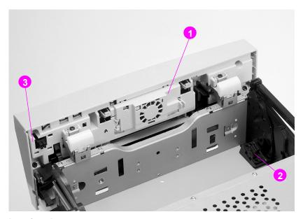
Figure 7-33 Imaging drum connector
