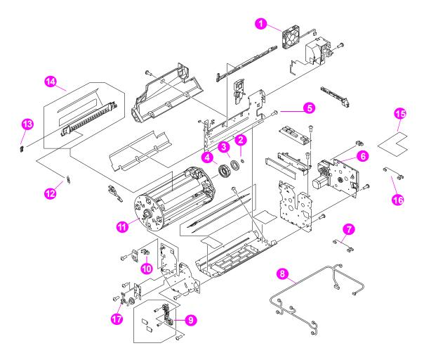
Figure 8-9 Developing carousel assembly
