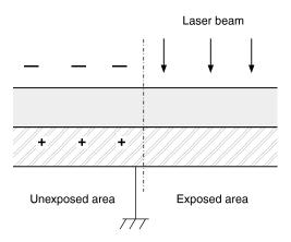
Figure 5-4 Laser exposure
