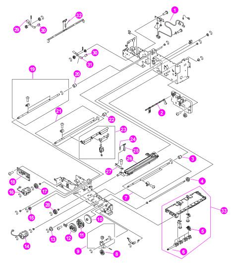
Figure 8-12 Paper pick-up assembly (3 of 3)
