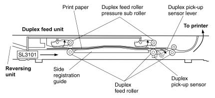
Figure 5-35 Duplex feed roller pressure
